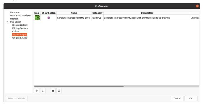
The KiCad PCB editor supports plugins written in Python that can perform actions on the board being edited. These plugins can be installed using the built-in Plugin and Content Manager (see the KiCad chapter for details) or by placing the plugin files inside the user plugins directory. See the Scripting section below for details.
